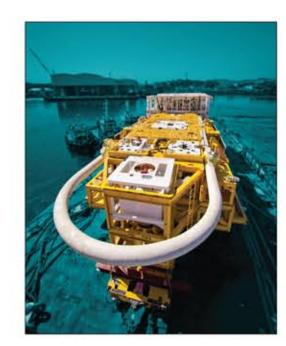
The Marlim subsea separation system was designed and manufactured for Petrobras by FMC Technologies. The system is shown on Fundão Island prior to its installation in approximately 2,950 feet (900 meters) of water in the Campos Basin, offshore Brazil. Marlim was designed to be the industry's first application of oil and water separation technologies in deep water, and it is also the first system to separate heavy oil and water and to reinject water into a subsea reservoir to boost production.
